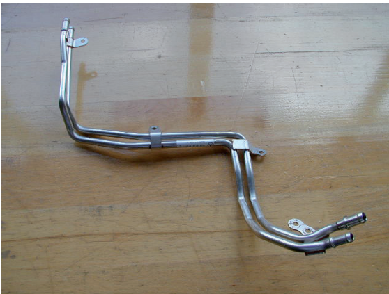
Picture 3 - Finished fuel lines
