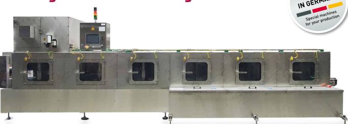
Our washing tunnel reliably removes lead dust, acid and other possible contamination. The extra powerful fan in combination with the heater ensures absolutely dry batteries.
