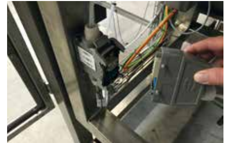
Once the base plate arrives at the front limit stop the quick release clamps can be attached and the modular plug connected. The changing cart can be removed and the machine is ready to produce with a new plug type.
