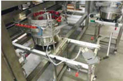
The changing cart can be moved to the frame with the required vibration feeder and pushed in.
