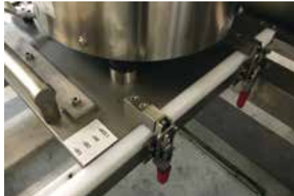
Once the base plate arrives at the front limit stop the quick release clamps can be attached and the modular plug connected. The changing cart can be removed and the machine is ready to produce with a new plug type.
